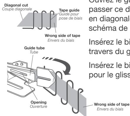
Pull 2" (5 cm) of the tape out of the muzzle of the tube, and fold the tape at a right angle.
